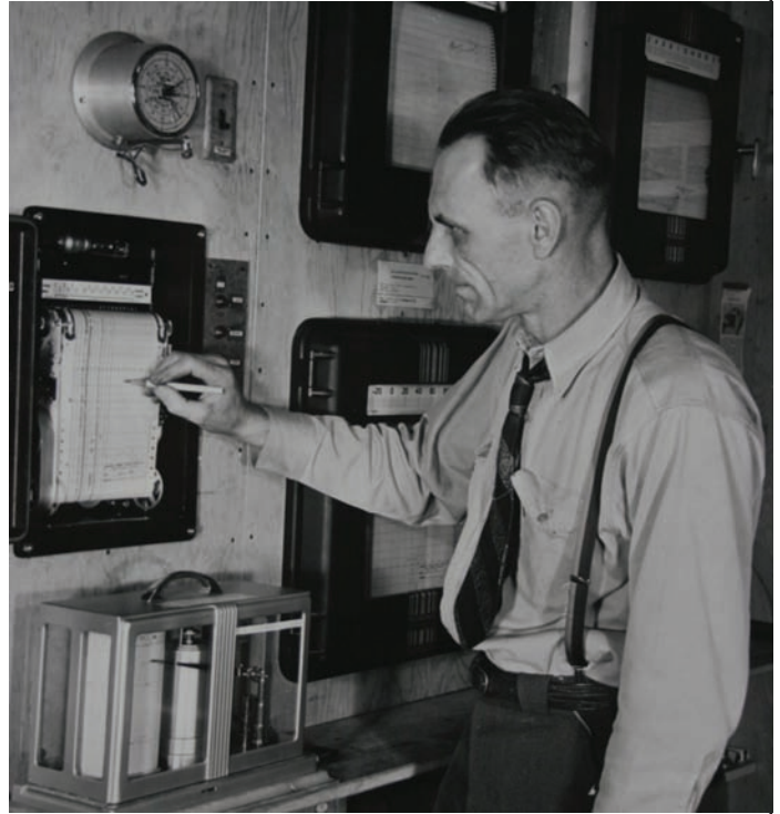
Above: Dr. Robert Gerdel, CSSL instrument panel. Triple register modified from Esterline-Angus recorder. Records velocity and direction of wind and duration of sunshine. It can handle twenty instruments. March, 1946
