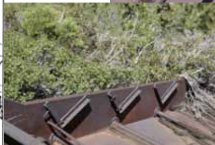
More of the Cisco boat tow. Above the bench supports, the wood has rotted away.
