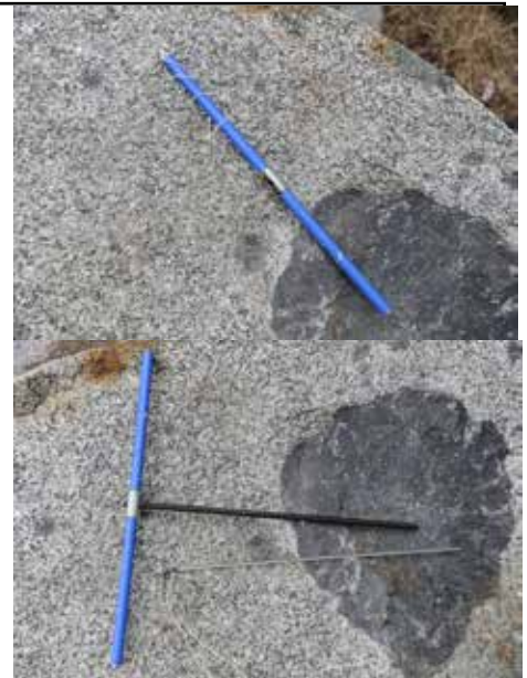
Dick Fores' incremental borer. Top picture shows the closed tool; bottom picture shows it ready for use. The borer is screwed into the tree and the thin "scoop" (the long thin metal thing below the borer) is inserted in then, pushed in and then the borer is rotated. The "scoop" is withdrawn pulling out a core. The core is then stored in a straw.
