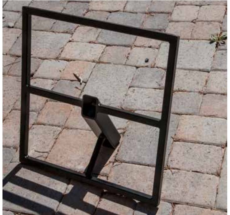
Here's the beautiful new removable top frame. We can just slip this onto the upright for summer and slip it off for winter.
