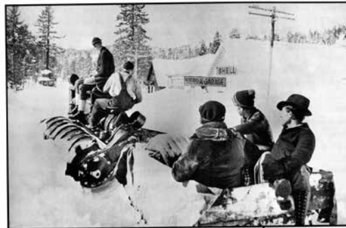
In the mid 1930s, Truckee resident James McIver, Jr. built a prototype snowmobile from a kit that adapted a Fordson Tractor power plant for traveling through snow. McIver’s “Snow Devil” utilized two long rotating drums with raised screw threads welded to its surface. The two rotors were chain driven to “screw” their way through the snow. McIver’s rig could only travel up to five miles per hour, but it effortlessly hauled supplies and passengers on a sled it pulled behind. (Courtesy Truckee Donner Historical Society.)
